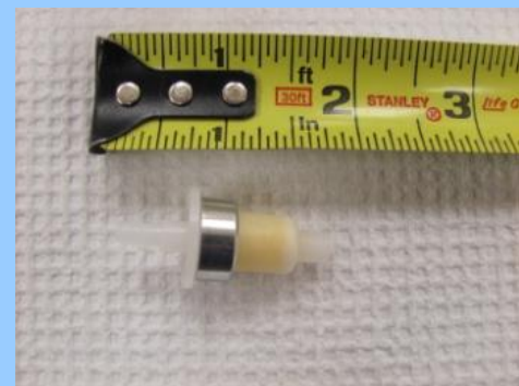
2, 4 - Dinitrophenylhydrazine (DNPH) cartridge sampling for carbonyls
