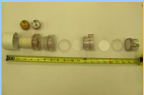
Filter pack sampling for PM 2.5 and precursor gases
