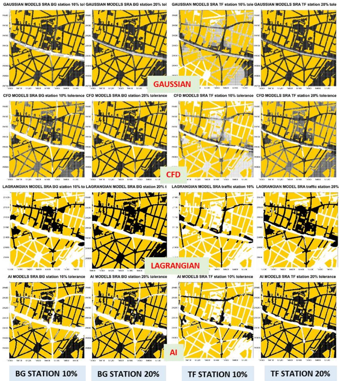
Figure 2. Overlapping of the spatial representativeness areas computed by the different types of model applications for the background (left) and traffic station (right) and for 10% and 20% tolerances. The darker the pixel, the more models estimate it is within the area of exceeding the limit value. The white color pixel indicates none model predicts it within the SRA.
