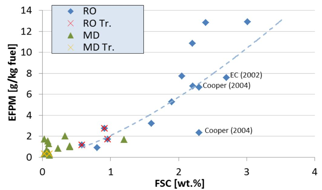
Emission factors for particle mass EFPM as a function of FSC (in wt. %). EF(PM) for RO is plotted in blue, EFPM for MD is plotted in green. Datapoints with crosses (Tr.) are from the Transphorm measurement campaigns.
