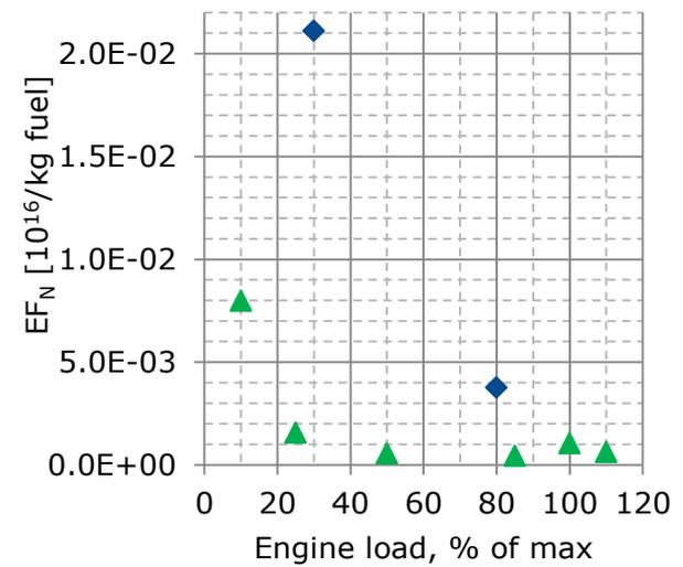
EF(PN) measured on test engine burning RO with FSC 2.21 (test engine), and 0.91 (Tr1) and in airborne measurements in ship plumes. a – total and non-volatile particles, b – particles in accumulation mode. (from Petzold et al., 2010, D2.1.4 and Jonsson et al., 2011)
